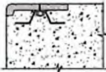
Style B-1 with wing anchor set into poured in place concrete. See page 2.
