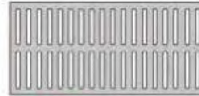
Type "HH" Grate (slots run perpendicular to frame. Slots to 5/16" wide for pedestrian traffic.)
