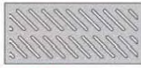
Type "AAA" (slots run diagonal to frame. For handicap/bicycle safety.)
